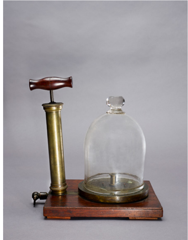
Vacuum pump with bell jar, ca. 1800–1850, Division of Medicine and Science, National Museum of American History, Smithsonian Institution
